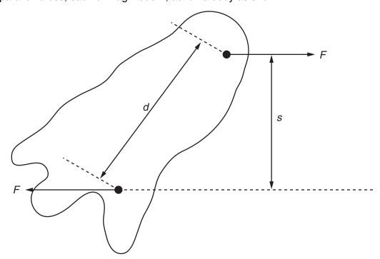
What is the magnitude of the torque on the body produced by these forces?
